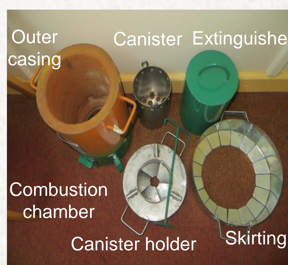
Top Lit Up-Draft (TLUD) gasifier, produced in Kenya
